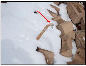
Figure 18: Sharp bend in wall tie where it was bent downward within void of CMU
