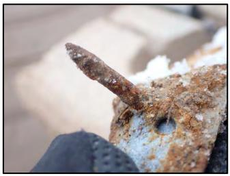
Figure 22: Corroded PAF
